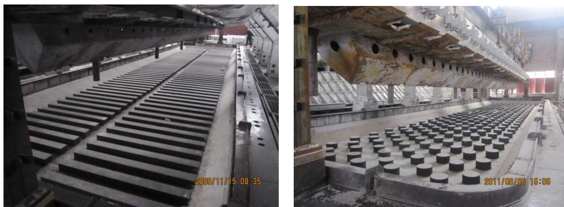
Figure 3. Industrial aluminum electrolysis cells installed with the novel structure cathodes (NSC). Left picture: cathodes with “raised” transverse ridges; right picture: cathodes with “raised” small cylindrical columns.
